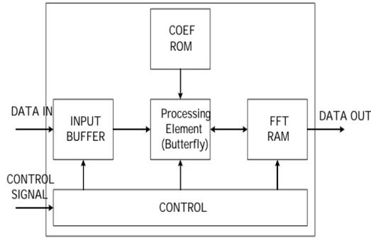
Fig1. Internal architecture of FFT/IFFT processors
