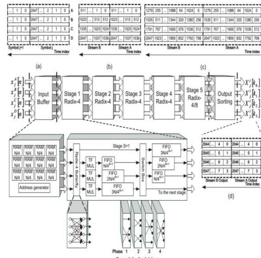
Fig. 2. Block diagram of the proposed MIMO MDC FFT/IFFT processor. The routing rule updates every  $N/4s+1$  clock cycles. (a) Initial input order. (b) Sorted input order at the output of input buffer. (c) Computed output order without sorting. (d) Output order after output sorting
